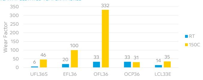
ASTM3702- mod. @ 50 fpm, 40psi \* Wear factor [10<sup>-10</sup> . in<sup>5</sup> .min/ft.lb.hr]
